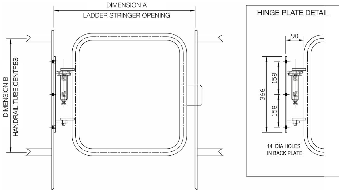
HINGE DETAILS - ALL FITTINGS TO BE FULLY WELDED TO GATE. HINGE PLATE TO BE BOLTED TO LADDER STRINGER.
